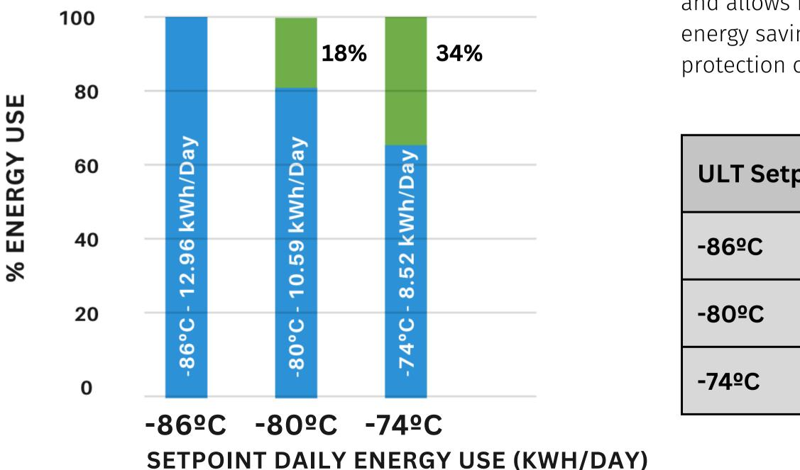
A brand new, state of the art ULT freezer uses much less daily energy, but still has only 4 hours of warm up time during power interruption. As a result, many freezers are kept at -86°C.
